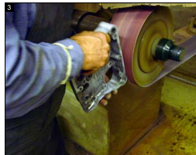
3 Initial polishing stage: parts are machine-belt sanded.
