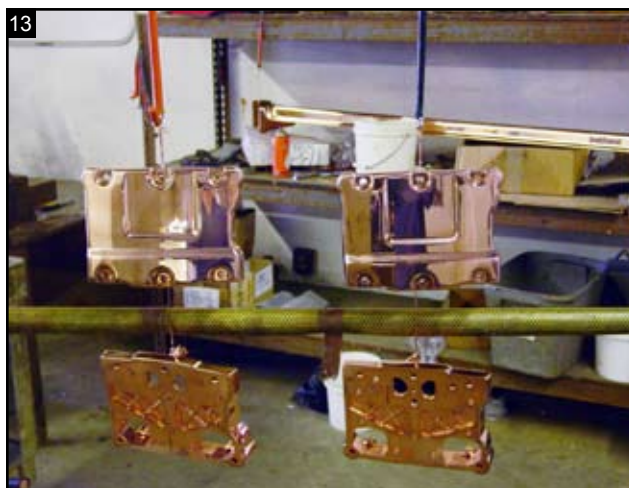
They're now ready for a final nickel layer and a chrome bath.
