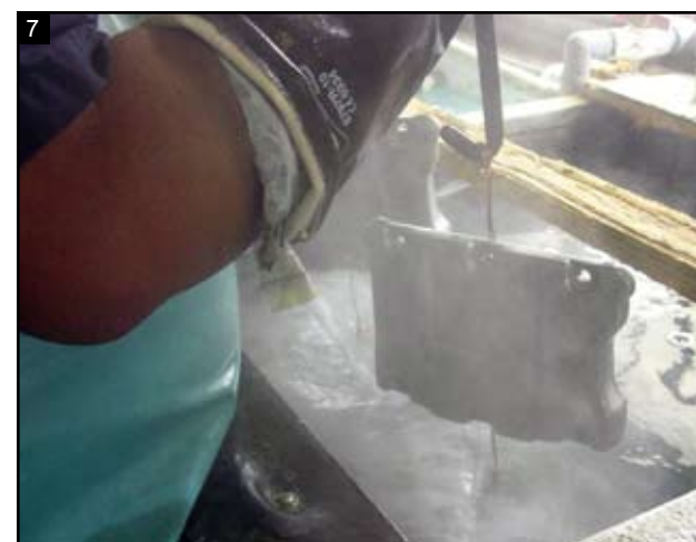
7 Parts are removed from the electro cleaner and ready for nickel plating.
