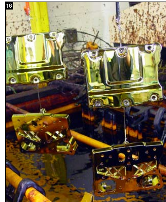
And lastly, the parts receive a chrome-plating bath.
