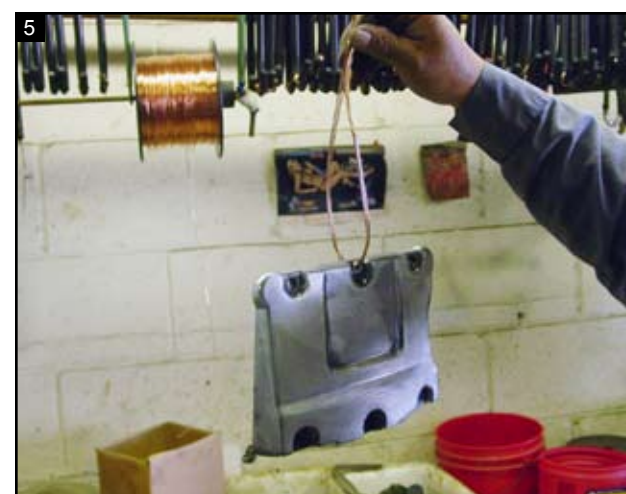
5 Parts are racked for initial copper strike (plating).
