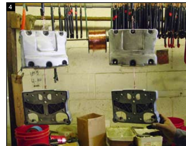
4 Parts are polished, rinsed and ready for copper strike.
