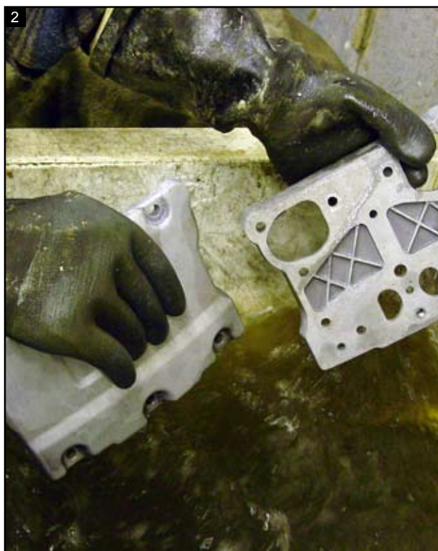
2 Parts are stripped of their paint or anodize.
