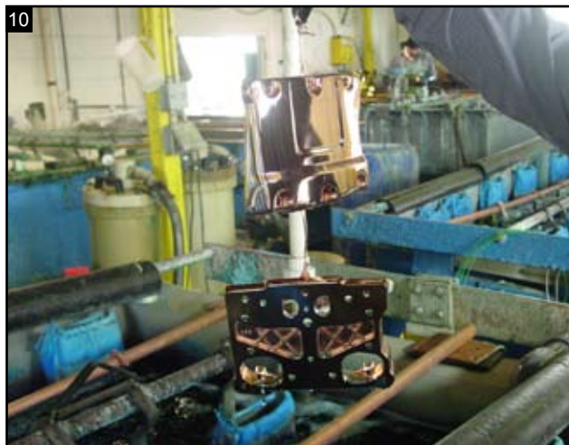
Parts after the acid copper bath.
